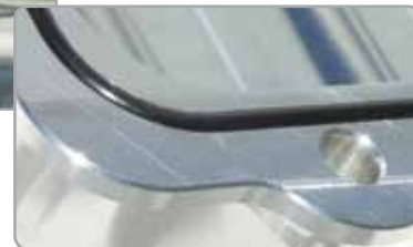
O-ring groove in fully machined pan rail
