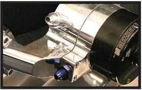
inlet side (the polished fitting toward the back of the pump). This will offer both connections for your transmission pan plumbing.
