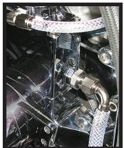
This photo shows one possible location for the low pressure return into the tank of a "200" style Meziere water pump.
