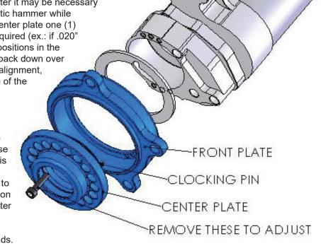
Step 6: Install the starter and check final clearances. If more adjustment is necessary repeat steps 1 through 6.
